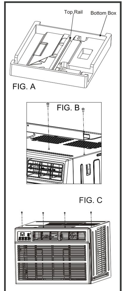
**NOTE:** For safety reasons, all 4 screws must be used to attach the top rail.
