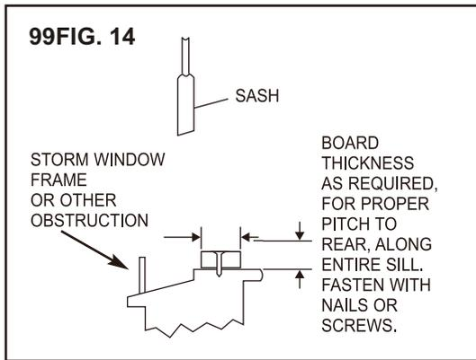
If Storm Window Frame must remain, be sure the drain holes or slots are not caulked or painted shut. Accumulated Rain Water or Condensation must be allowed to drain out.
